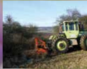
Clearing shrubs with the mulcher.
